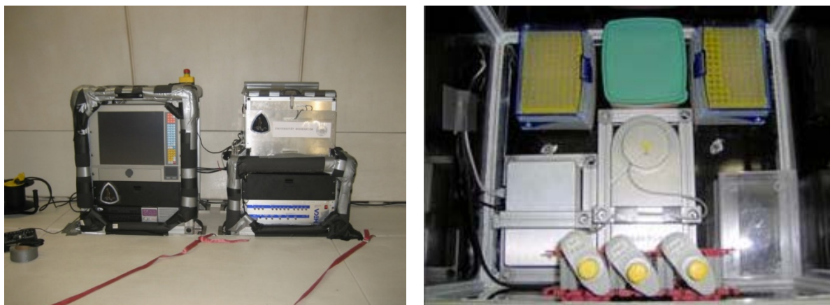
Figure 1. Semi automated patch-clamp (bilayer) set up for parabolic flights based on a Nanion Port-a-Patch system in flight configuration. The patch-clamp set-up itself (right) and the data acquisition system (left) are placed in separate flight racks. 19-inch-rail components have been used. The photo on the right shows the interior of the experimental chamber.
